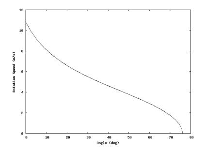
If the walls are vertical ( $\theta = 0^{\circ}$ ) the rotational speed needed is about 10.84 m/s and as the angle increases (the walls start tilting over), the speed needed gradually reduces but then something odd happens at high angles. The speed needed drops to **zero** at about  $\theta = 76^{\circ}$ . What's happening there?
