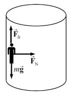
Let's use Newton's Laws to analyze this situation and determine how fast the ride needs to rotate for this to work.
