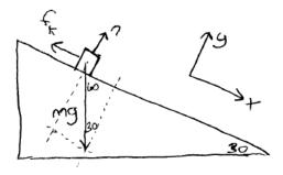
Friction and the normal force are already aligned with one of the coordinate axes, but  $F_g$  is not, so we'll need to get its components. Moving the angles around, we find a right triangle we can use to determine the components of  $F_g$ . Here, we see that the weight has a component down-slope of  $mg \sin 30$  and a component in the -Y direction of magnitude  $mg \cos 30$ .
