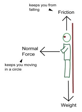
Let's look at the edge case though: suppose we only have **just enough** static friction to hold the person in place, with nothing left over. So we're looking at the case where  $f_s = f_{s,max} = \mu_s F_N$ .
