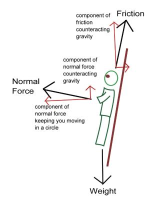
Let's use a coordinate system where one of the axes is in the direction of the acceleration vector (so radially inward) and then the other axis has to be perpendicular to that so let's use a Y axis with +Y vertically upward.
