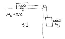
(a) Verify that the present situation is stable (i.e. static friction is providing enough force to keep the trailers from sliding over the edge).
