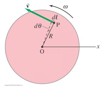
Shrinking the time interval down, we get the calculus limit version of instantaneous angular velocity:
