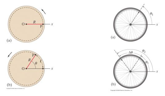
(a) As an object rotates, every point on that object rotates through the exact same angle  $\theta$ .
