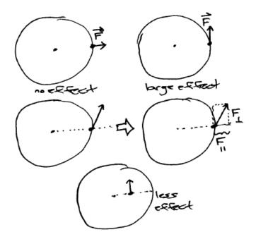
The angular acceleration is proportional to r (how far out from the axis the force is applied), and is also proportional to the component of the force tangent to  $\vec{r}$ .
