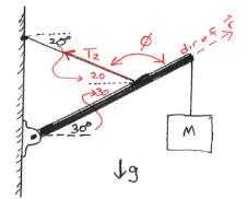
The  $\phi$  that we need is marked in the figure, so that angle must be  $180 - 50 = 130^{\circ}$ .
