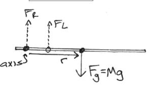
Using the RHR or looking at how this single force would cause the pole to rotate about the axis we chose, the pole would rotate clockwise about that point, so this torque will be negative. Finally:  $\tau_{F_g} = -(1.6)(Mg)$ .
