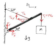
In the Y direction, we have the wall force  $F_y$ , the Y component of  $T_2$  (up), and the 196 N of tension in  $T_1$  (down), so:
