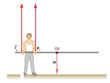
**Newton**: To apply Newton's Laws, let's define our coordinates to be +X to the right on the page, and +Y vertically upward (i.e. towards to the top of the page). Then  $\sum F_y = ma_y = 0$  implies that  $F_R + F_L - Mg = 0$  or  $F_R + F_L = Mg$ . (Remember, we're starting off assuming both  $F_L$ and  $F_R$  are positive upward and we'll just let the algebra tell us what direction they're really in.)
