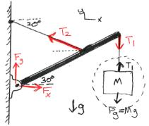
We can immediately determine tension  $T_1$  though by applying Newton's Laws to another object: the hanging sign itself.  $\sum F_y = 0$  on the sign so  $T_1 - mg = 0$  or  $T_1 = mg = (20 \ kg)(9.8 \ m/s^2) = 196 \ N$ .
