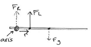
Using the RHR, we see this will be a positive torque. (Or: if we force the pole to rotate about our chosen axis and then apply just this force, which is upward on the page, that will cause the pole to rotate counter-clockwise, making this a positive torque.) Finally:  $\tau_{F_L} = +(0.6)(F_L)$ .
