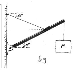
Note: the point where the pole is connected to the building is a swivel joint with frictionless ball bearings, so the point won't introduce any torque.)
