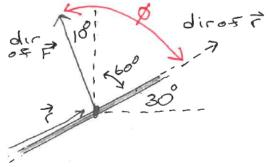
Collecting terms:  $\sum \tau = 0 + 0 - 84870 + (15)(F_T) \sin(70^\circ)$  which leads to  $F_T = 6021 N$ . (That's quite a bit less tension in the cable than we needed in the previous version.)
