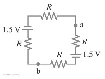
5. For the circuit shown, find the potential difference between points (a) and (b). Each resistor has  $R = 130 \ \Omega$  and each battery is 1.5 V.
