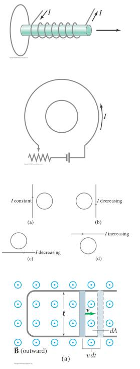
• HW 29.08 : (a) If the resistance of the resistor in the figure is slowly increased, what is the direction of the current induced in the small circular loop inside the larger loop? (b) What would it be if the small loop were placed <u>outside</u> the larger one, to the left? Explain.
