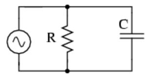
At the given frequencies, what is the impedance of the resistor? The capacitor? The elements are in parallel, so will have the same  $V_{rms}$  across each of them and  $V_{rms} = I_{rms}Z$  for each. We don't know  $V_{rms}$  here, but it's the same for each, so we can at least relate the different  $I_{rms}$ values through each element for each of the two different frequencies.
