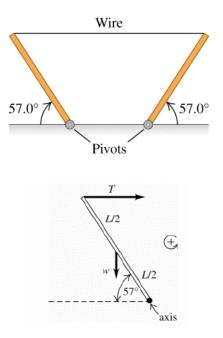
The wire has a mass per unit length of  $\mu = M/L = (0.732 \ kg)/(5.00 \ m) = 0.146 \ kg/m$ . Waves on this wire then will propagate with a speed of  $v = \sqrt{F/\mu} = \sqrt{(76.3/0.146)} = 22.86 \ m/s$ .
