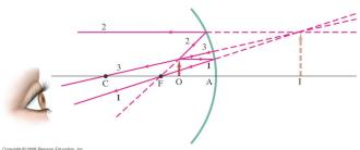
Here we have a 1 cm tall object placed 10 cm from a concave mirror that has a radius of curvature of 30 cm. Let's follow three of the many photons spewing out from a point on the object.
